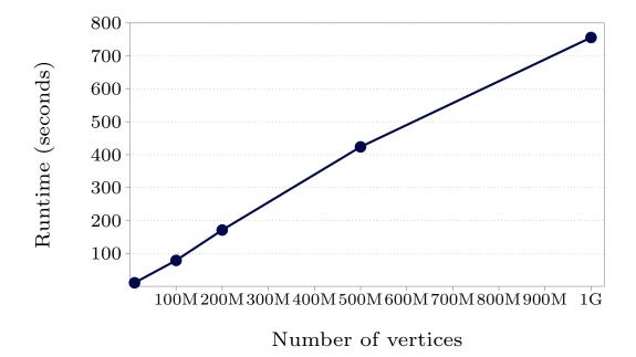
Figure 9: SSSP—log-normal random graphs, mean out-degree 127.1 (thus over 127 billion edges in the largest case): varying graph sizes on 800 worker tasks scheduled on 300 multicore machines
